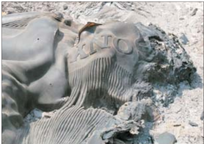
Molten television. Use of brominated flame retardants and heavy metals in plastics by manufacturers such as Sony create very dangerous emissions when burned and disposed in this way. © BAN
