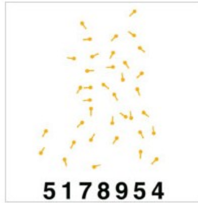
The minutia are converted via an algorithm and saved as reference template.
